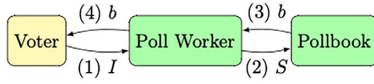
Figure 2: Example ProveRegistration flow. Here, G = \text{Poll Worker} and G' = \text{Pollbook} . All communication channels are in person.
